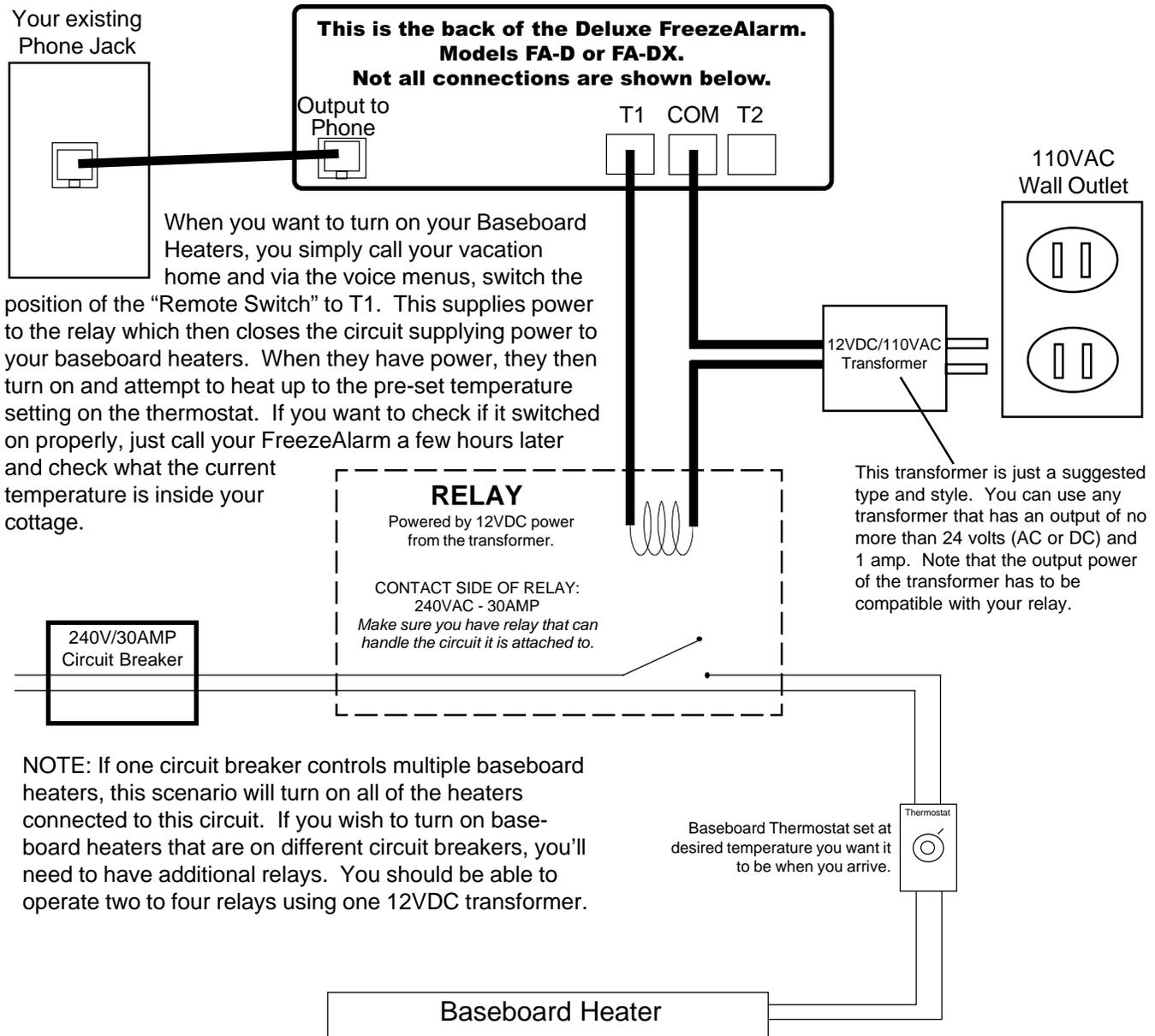
NOTE: If one circuit breaker controls multiple baseboard heaters, this scenario will turn on all of the heaters connected to this circuit. If you wish to turn on baseboard heaters that are on different circuit breakers, you'll need to have additional relays. You should be able to operate two to four relays using one 12VDC transformer.
